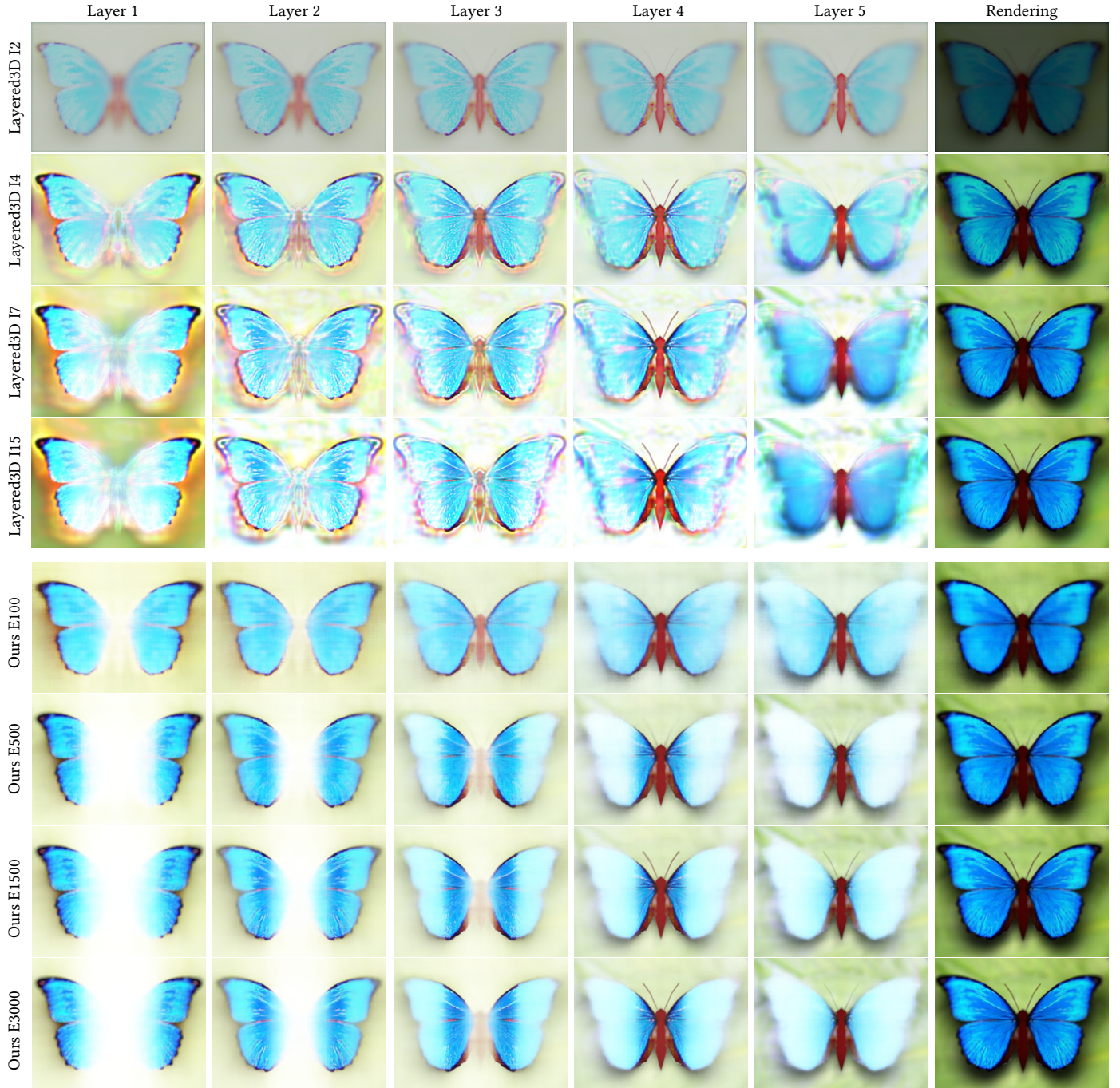
Fig. 8. Comparisons of transmission maps from Layered3D (upper four rows) and our approach (lower four rows). The thickness of the display is 12.5 mm. The rightmost column shows the rendered test views.
