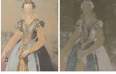
Fig. 16. Image marked on AISI 304 and captured in non-diffuse (left) and diffuse (right) modes. Painting © Alessandro Allori.
