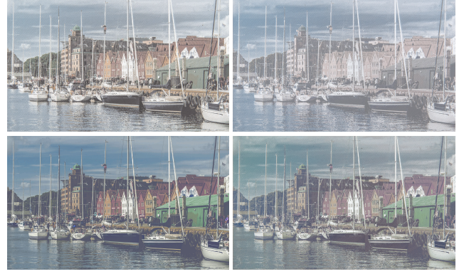
Fig. 14. Marked images on AISI 304 (top left) and AISI 430 (top right) with the same primaries explored and extracted on AISI 304. A newly explored and extracted set of primaries on AISI 430 are used for marking an image: gamut-mapped (bottom left) and photograph (bottom right). Image © Piotr Didyk.
