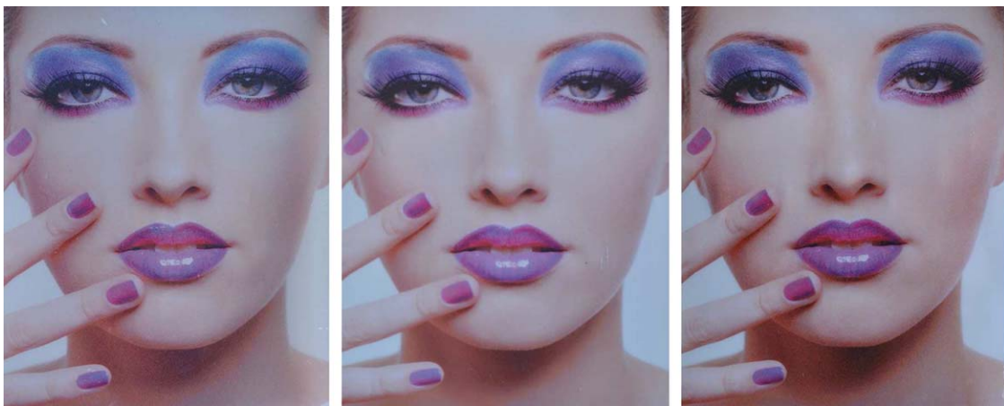
Fig. 8. Center: the photograph of an original print without deformation. Left: the printed image after 45% of shrinking created with our custom color reproduction framework. Right: the printed image after 45% of shrinkage without any compensation.
