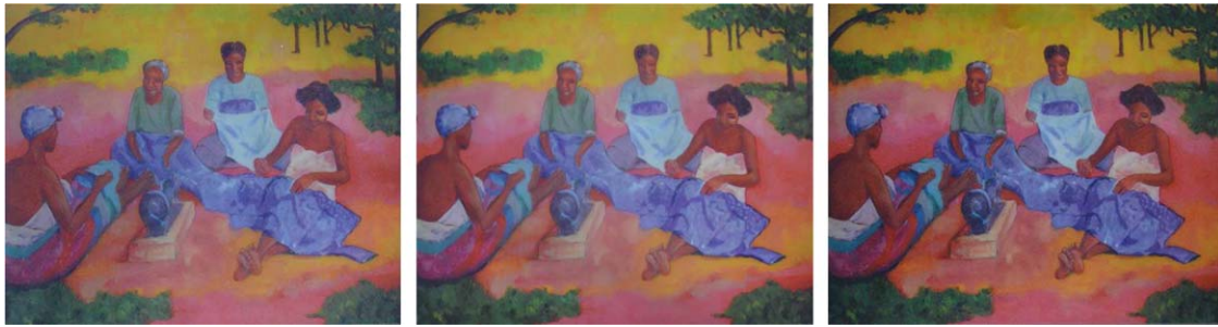
Fig. 7. Center: the photograph of an original print without deformation. Left: the printed image after 61% of shrinking created with our custom color reproduction framework. Right: the printed image after 61% of shrinkage without any compensation.
