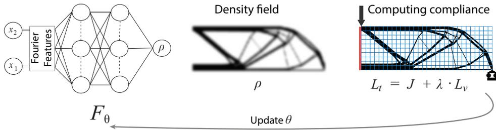
**Figure 1: A single iteration of our end-to-end differentiable topology optimization via explicit design representation networks.**
