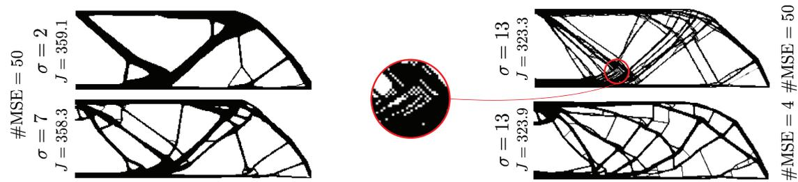
**Figure 10: Results from our experiments using density-space OC to train ENDR. While parameter  $\sigma$  retains some control over the design's complexity (left), it is much less effective and significantly worse stiffness is achieved versus directly minimizing compliance with Adam; compare to Figure 2. These issues can be mitigated somewhat by limiting the number of fitting iterations (bottom right), but still most of ENDR's benefits are lost.**
