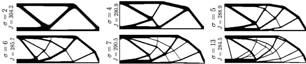
Figure 2: The effect of the scale hyperparameter  $\sigma$  on the quality and compliance (topology optimization of an MBB beam at  $300 \times 100$  resolution). The  $\sigma$  range shown here, at this resolution, produces a diverse set of designs beyond which we did not obtain novel solutions.
