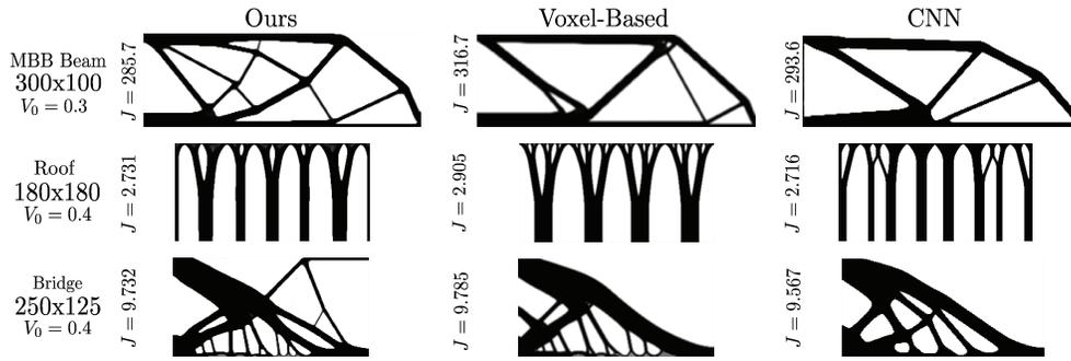
**Figure 6: Comparison of the proposed method against the voxel- and CNN-based methods for a set of boundary conditions. Our method produces qualitatively different results whose compliances are either very close to or below those from the other methods. In the middle row, for visualization purposes only, we have mirrored the final result of all models.**
