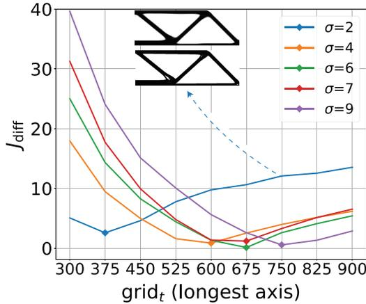
**Figure 5: We compute at a source resolution, here  $300 \times 100$ , a design, upsample it to different target resolutions (375, ..., 900), and use them as initializations for a standard voxel-based method. The smallest change in the compliance value indicates the best upsampling ratio for a source design.**
